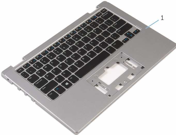
1 palm rest and keyboard assembly
